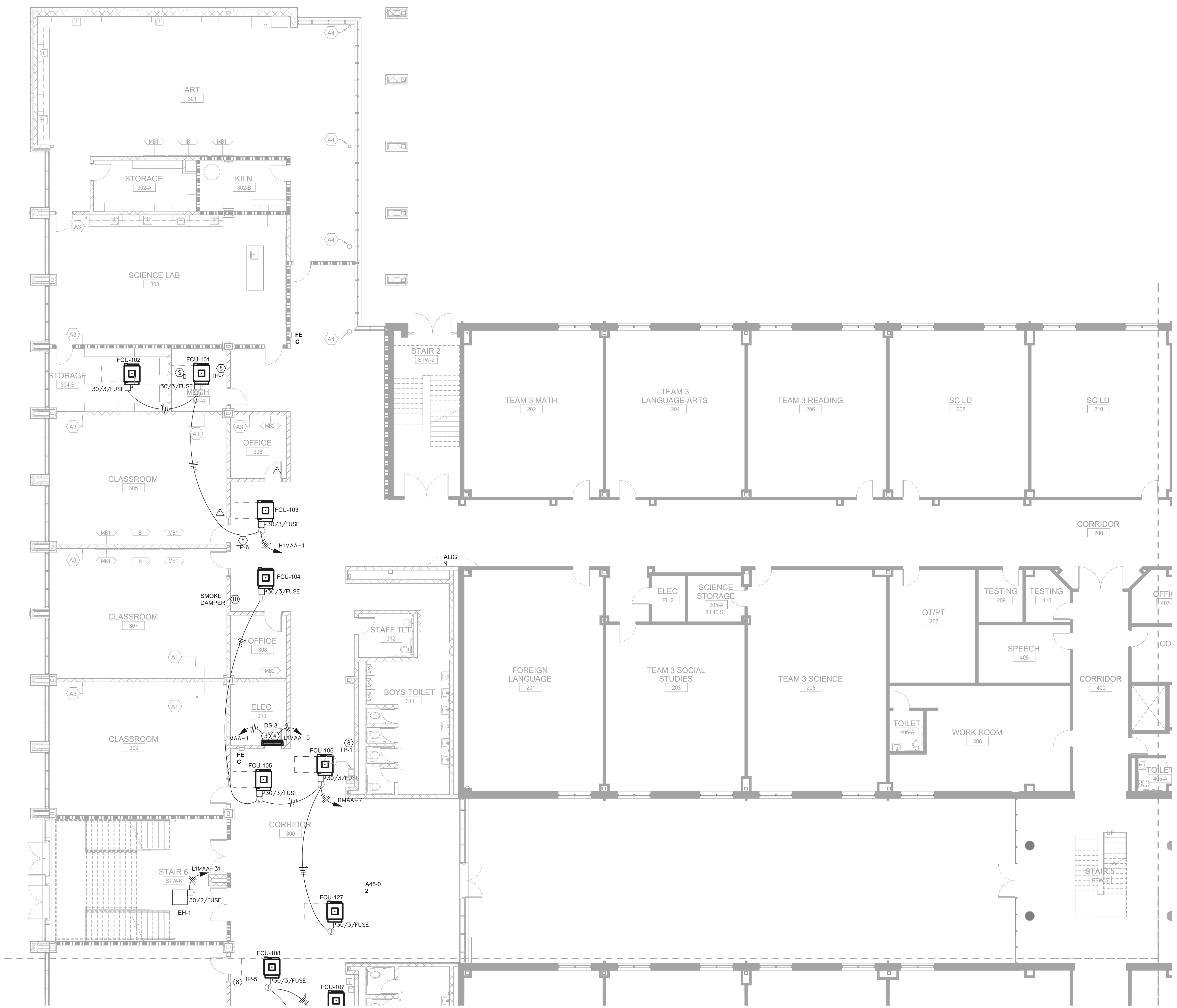
1 FLOOR PLAN - LEVEL 01 - AREA A - HVAC POWER 1/8" = 1'-0"
